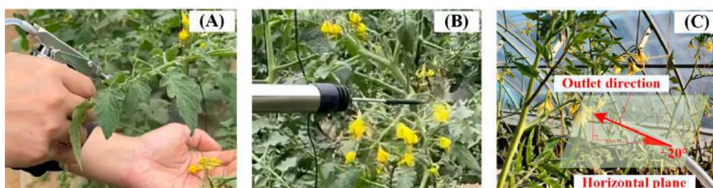
Figure 6. Operation scenarios of different assisted tomato fruit setting methods. (A) Assisted fruit setting with chemical agent spraying. (B) Assisted fruit setting with vibration pollinator. (C) Assisted fruit setting with pulse airflow pollination.
